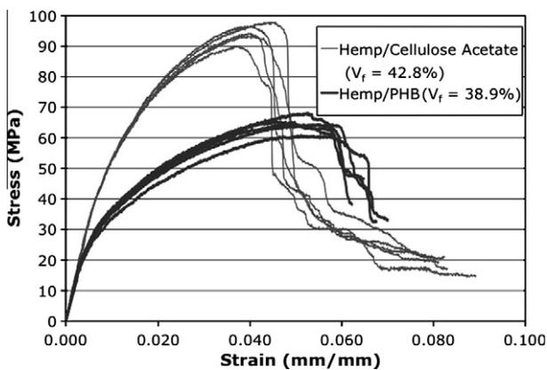
Fig. 4. Flexural stress–strain response of hemp/cellulose acetate and hemp/PHB composites.
