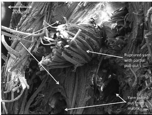
Fig. 2. Scanning electron image of hemp/cellulose acetate failure surface.
