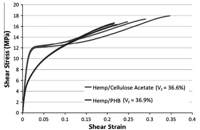
Fig. 3. Shear stress–strain response of hemp/cellulose acetate and hemp/PHB composites.
