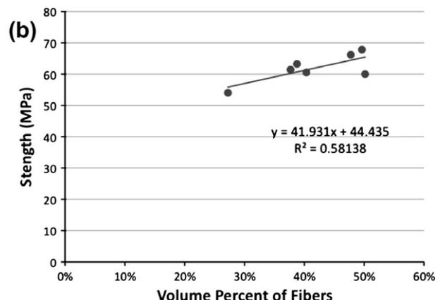
Fig. 5. Impact of fiber volume fraction on (a) tensile stiffness and (b) tensile strength.
