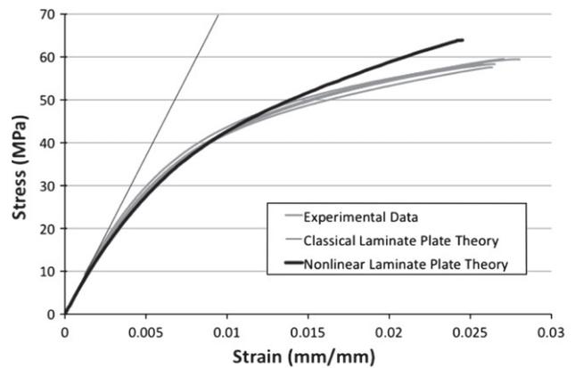
(a) Laminate 1T [0<sub>6</sub>/±45<sub>6</sub>/0<sub>6</sub>]
