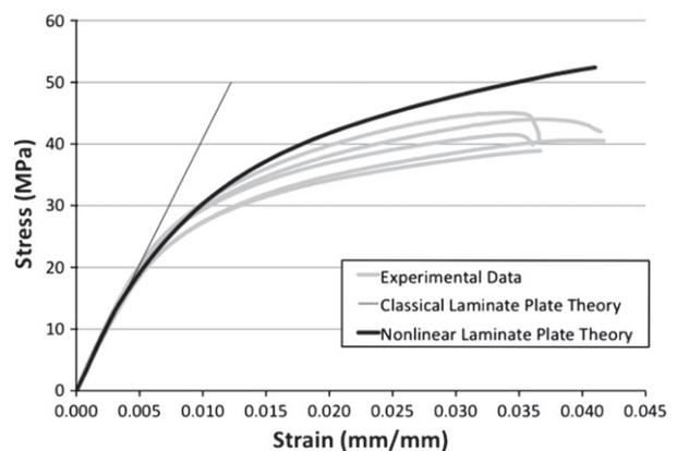
(c) Laminate 3T [0<sub>2</sub>/45<sub>2</sub>/−45<sub>2</sub>/90<sub>2</sub>]<sub>sym</sub>
