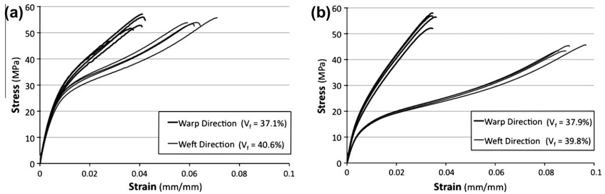
Fig. 1. Tensile stress–strain response for (a) hemp/cellulose acetate, and (b) hemp/PHB composites.
