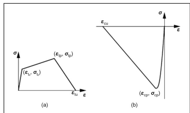
Fig. 6. Envelope curves for ECC constitutive model in (a) tension and (b) compression
