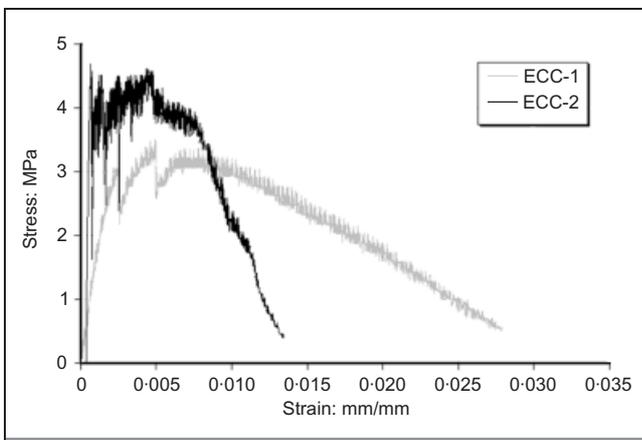
Fig. 3. Typical uniaxial tensile stress–strain behaviour of ECC mixes
