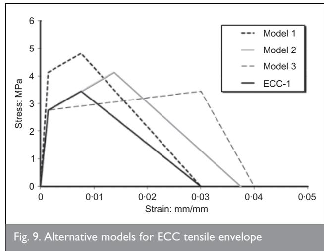
Fig. 9. Alternative models for ECC tensile envelope
