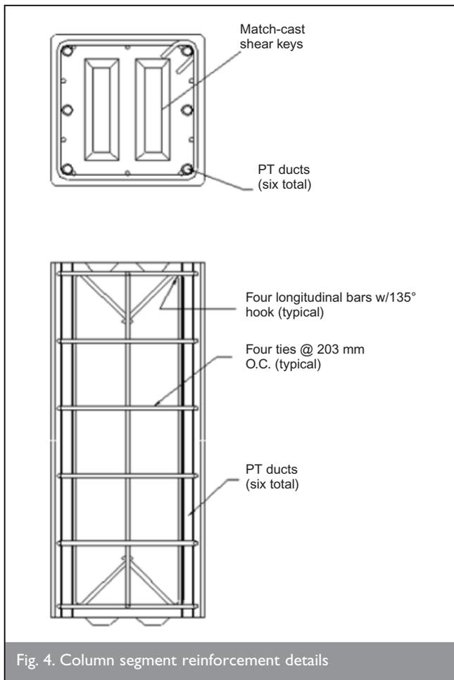
Fig. 4. Column segment reinforcement details
