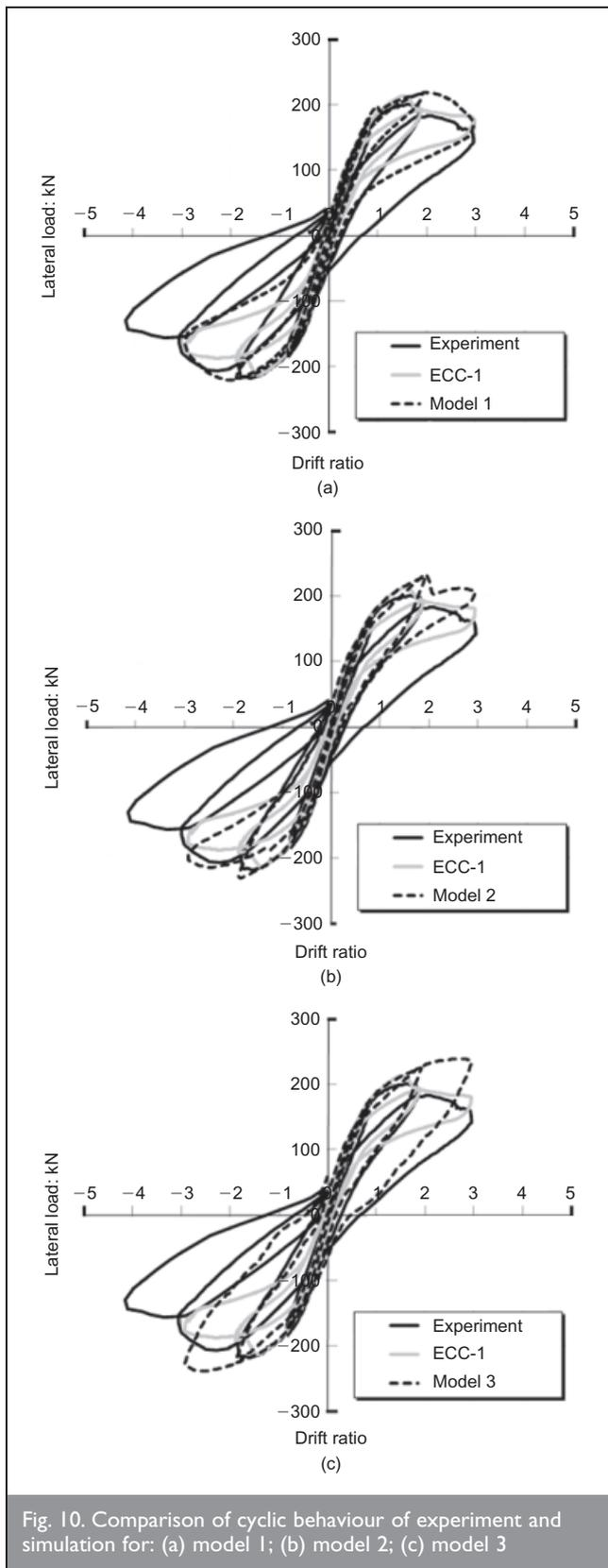
Fig. 10. Comparison of cyclic behaviour of experiment and simulation for: (a) model 1; (b) model 2; (c) model 3
