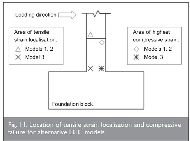
Fig. 11. Location of tensile strain localisation and compressive failure for alternative ECC models
