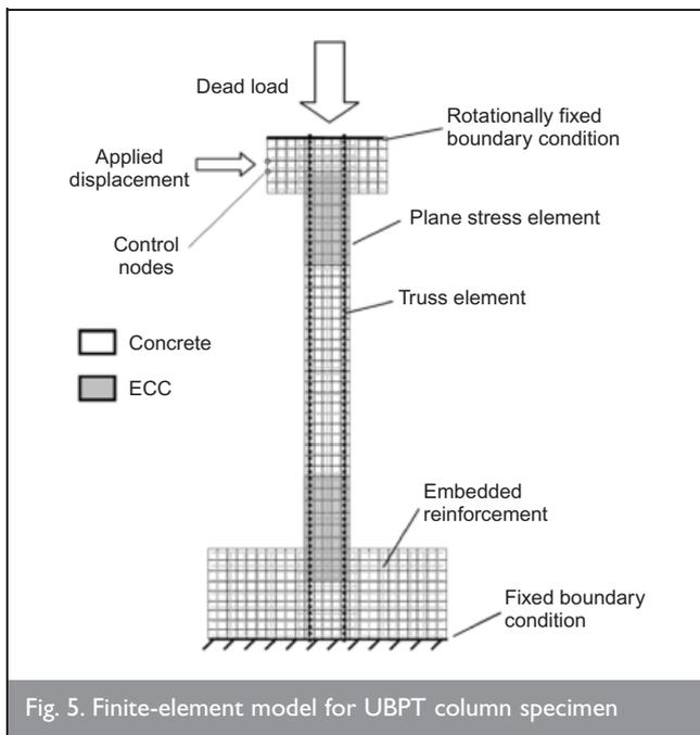
Fig. 5. Finite-element model for UBPT column specimen
