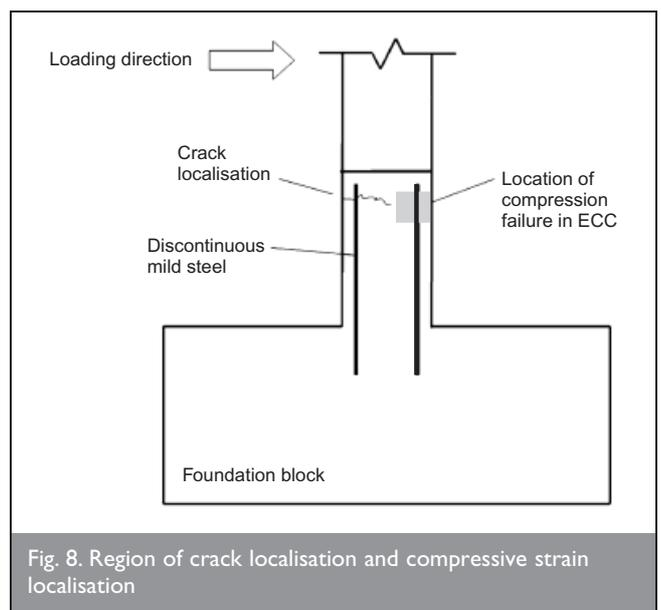
Fig. 8. Region of crack localisation and compressive strain localisation
