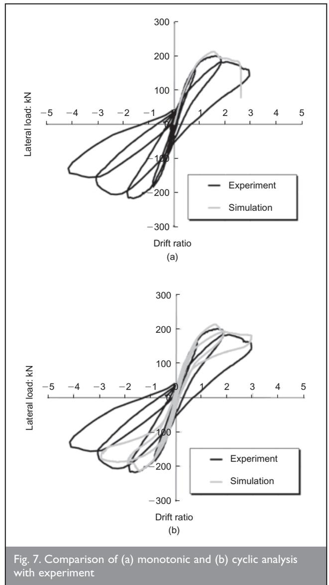
Fig. 7. Comparison of (a) monotonic and (b) cyclic analysis with experiment
