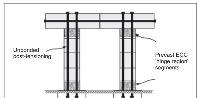
Fig. 1. Self-centring system bridge piers using unbonded post-tensioning to provide restoring force
