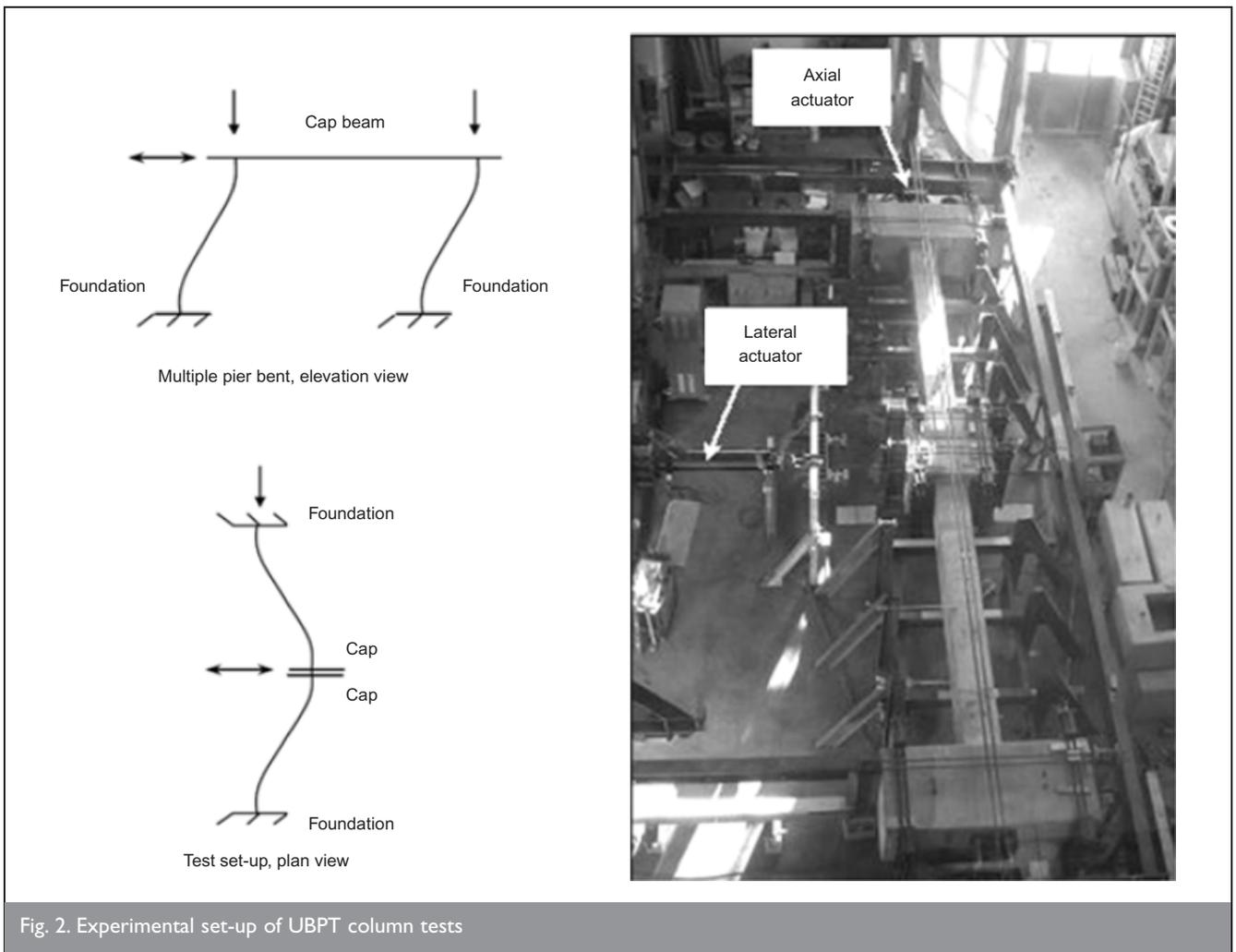
Fig. 2. Experimental set-up of UBPT column tests
