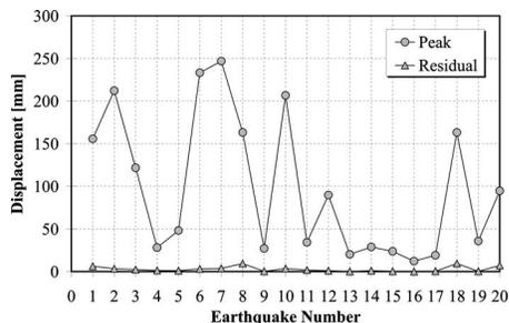
**Fig. 3.** Comparison of peak and residual displacements for fiber-element model subjected to near-fault ground motions
