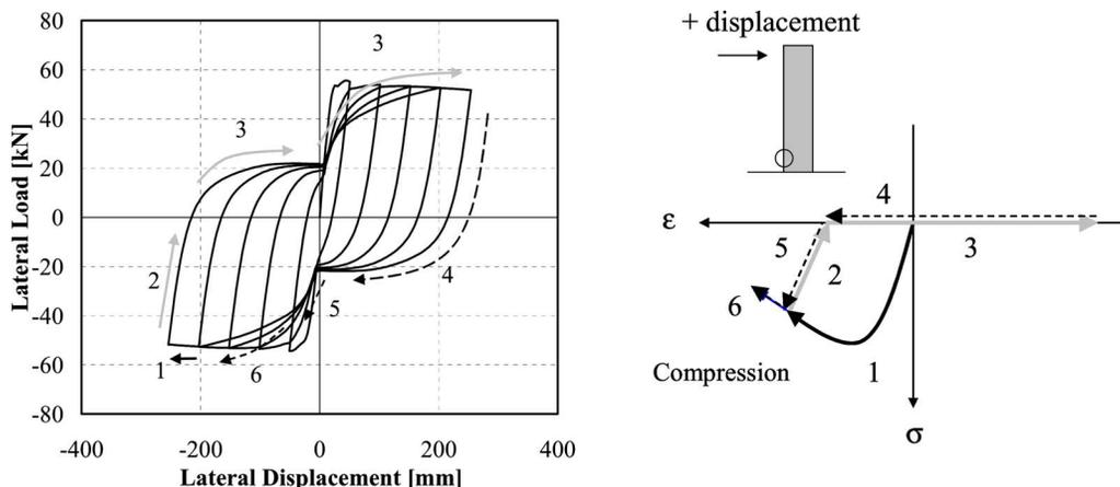
Fig. 9. Effect on (a) fiber-element model hysteresis from (b) constitutive behavior of concrete
