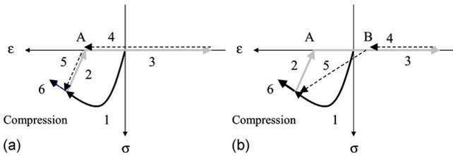
**Fig. 10.** Constitutive behavior of concrete in (a) unmodified; (b) modified model during unloading and reloading
