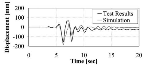
Fig. 2. Comparison of experimental and simulated displacement histories for RC column
