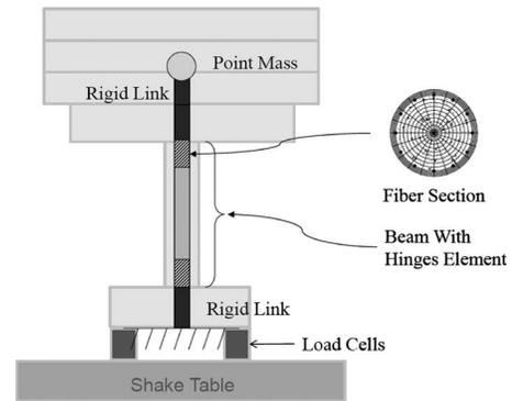
Fig. 1. Schematic of fiber-element model for RC column (adapted from Sakai 2005)
