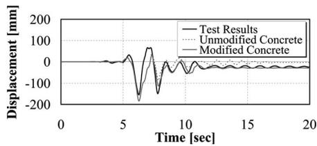
**Fig. 13.** Experimental and simulated displacement response histories using modified concrete model for RC column
