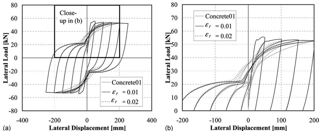
**Fig. 11.** (a) Load-displacement behavior of fiber-element model; (b) closeup view of SITC effect on hysteresis behavior
