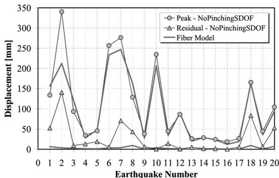
**Fig. 7.** Peak and residual displacement responses for NoPinchingSDOF model
