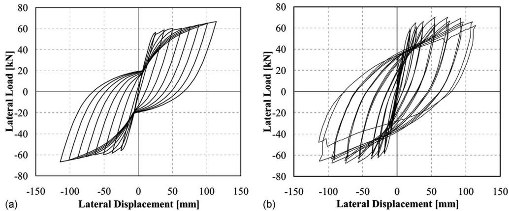
**Fig. 4.** Comparison of hysteretic response of (a) fiber-element model with no axial load; (b) experimental data (from Hamilton et al. 2002)
