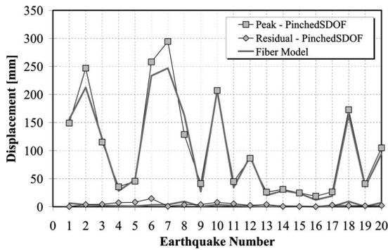
**Fig. 6.** Peak and residual displacement responses for PinchedSDOF model
