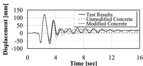
**Fig. 14.** Experimental and simulated displacement response histories using modified concrete model in the fault normal direction for RC column subjected to Olive view record
