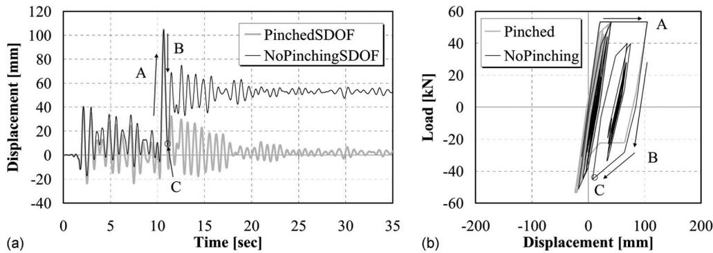
Fig. 8. Comparison of (a) displacement time history; (b) force-displacement response for SDOF models under earthquake Motion 20
