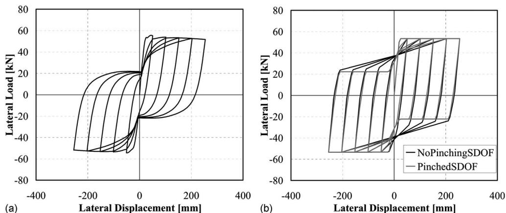
**Fig. 5.** Comparison of (a) fiber model hysteresis; (b) SDOF models
