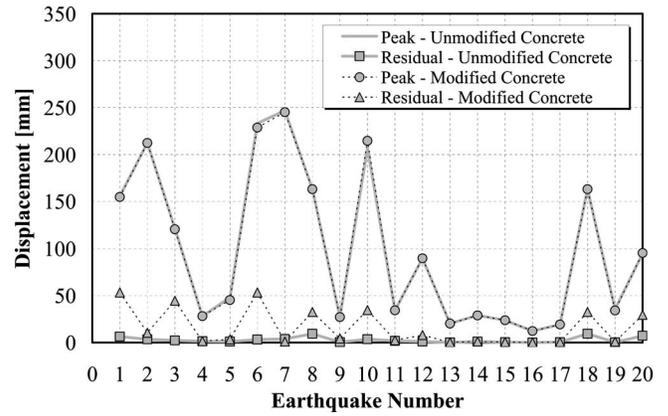
**Fig. 12.** Comparison of peak and residual displacement responses for fiber-element model with modified and unmodified models
