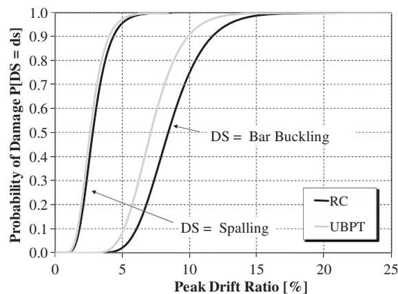
Figure 9. Fragility curves for spalling and bar buckling damage states.
