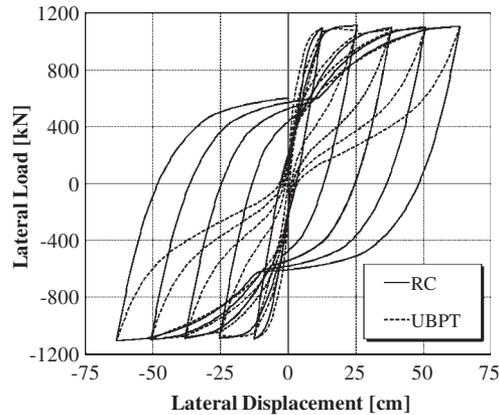
Figure 6. Cyclic analysis of RC and UBPT columns for baseline bridge.
