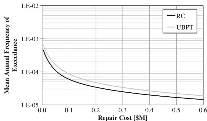
Figure 11. Hazard curves for peak-drift-related repair costs.
