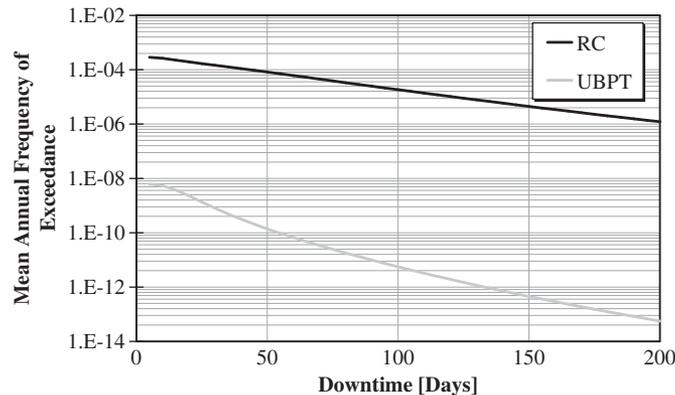
Figure 12. Hazard curves for downtime related to bridge demolition and replacement.
