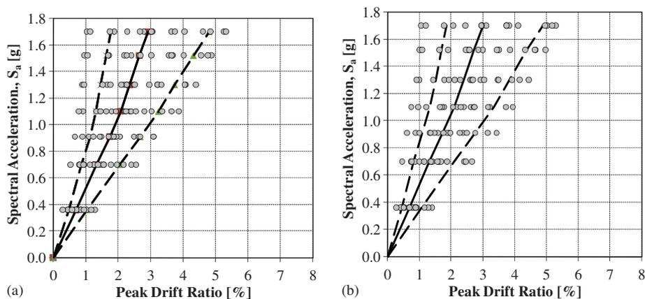
Figure 7. Comparison of peak drifts for bridge with (a) RC columns and (b) UBPT columns.
