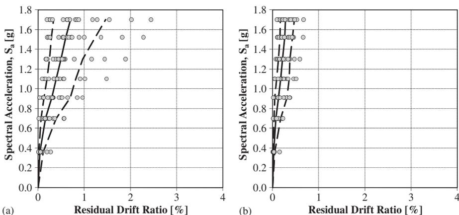
Figure 8. Comparison of residual drifts for bridge with (a) RC columns and (b) UBPT columns.
