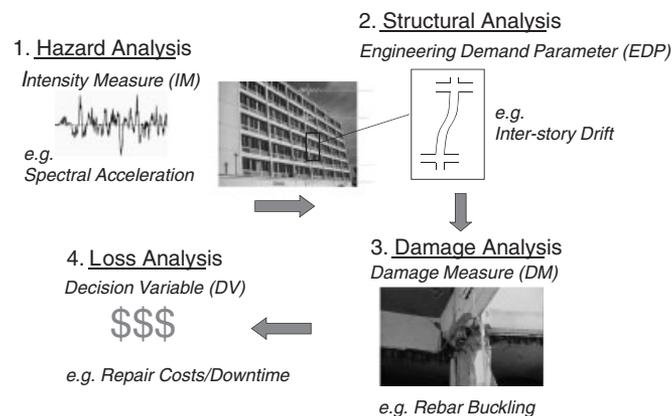
Figure 1. Performance-based earthquake engineering framework.
