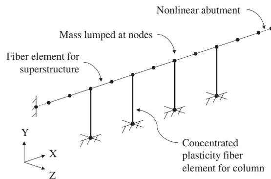
Figure 4. Schematic representation of bridge model.
