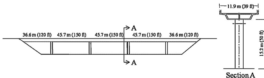
Figure 2. Bridge configuration and geometry.
