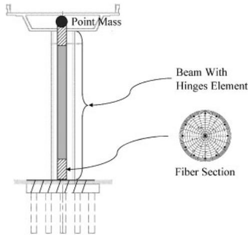
Figure 5. Schematic representation of column model.
