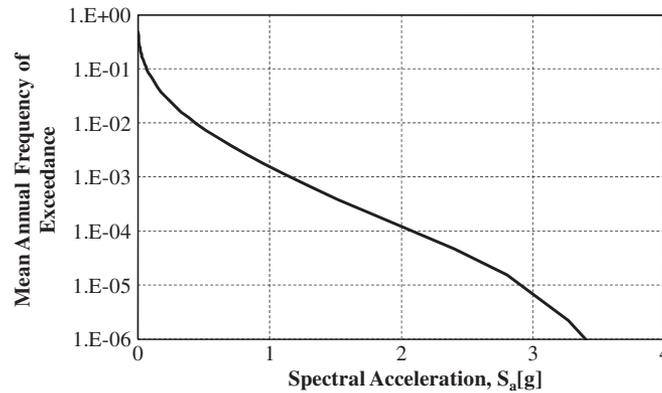
Figure 3. Spectral acceleration hazard curve for Oakland site.
