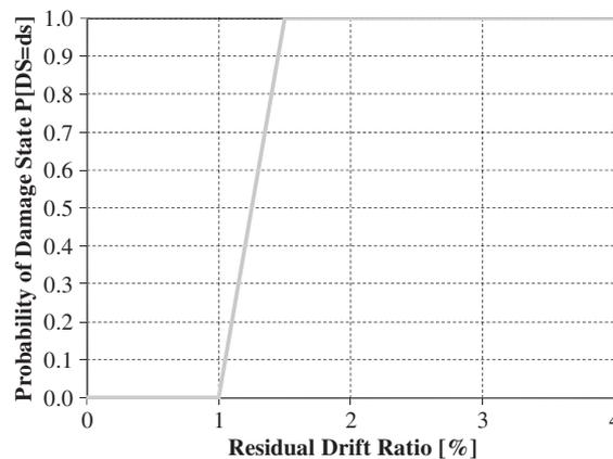
Figure 10. Fragility curve for excessive residual displacement damage state.
