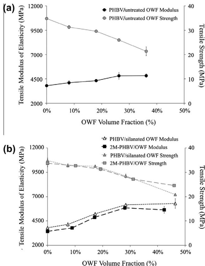
**Fig. 2.** Effect of (a) fiber loading and (b) fiber loading and chemical compatibilization technique on tensile modulus and tensile strength of PHBV/OWF composites. Each data point represents the average tensile properties of three (3) specimens. The error bars represent  $\pm$  one standard deviation.
