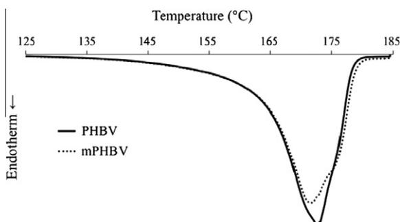
**Fig. 6.** Dsc thermograms for PHBV and mPHBV at a heating rate of 3 °C/min.
