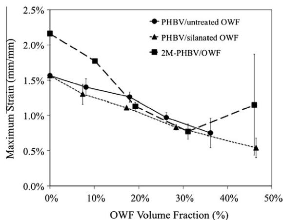
**Fig. 3.** Effect of fiber loading and chemical compatibilization technique on elongation to break of PHBV/OWF composites. Each data point represents the average tensile properties of three (3) specimens. The error bars represent  $\pm$  one standard deviation.
