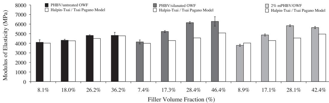
Fig. 7. Comparison of experimental results with the Halpin–Tsai/Tsai–Pagano micromechanical model for composite stiffness. The error bars show  $\pm$  one standard deviation.
