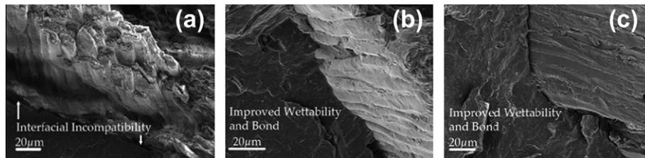
**Fig. 5.** SEM micrographs showing (a) the incongruous neat PHBV/untreated OWF fiber–matrix interface and improved fiber wettability achieved with compatibilization in (b) neat PHBV/silane-treated OWF and (c) mPHBV/untreated OWF.
