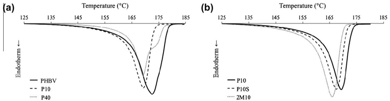
**Fig. 4.** DSC thermograms demonstrating the effect of (a) increasing OWF content on neat PHBV polymer and (b) compatibilizing 10 vol% PHBV/OWF composites with silane and MA on heat of melting. The scans were performed at a heating rate of 3 °C/min.
