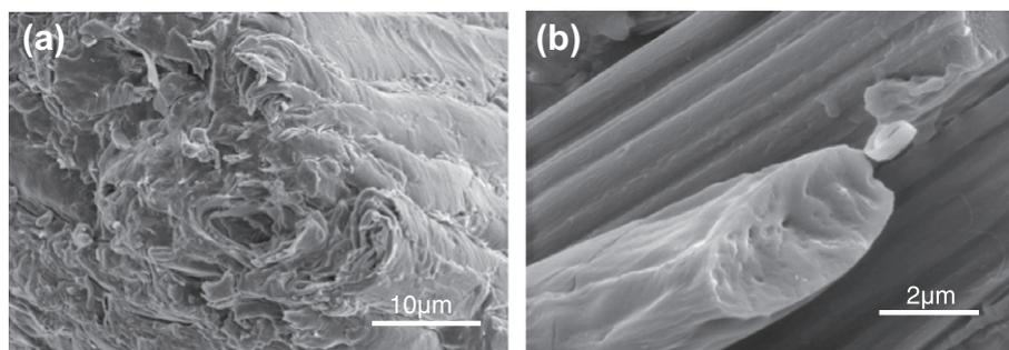
Fig. 1. SEM images of (a) collapsed wood fiber and (b) PHBV-filled lumen after fiber pullout.
